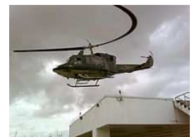
Distortion caused by a rolling shutter
